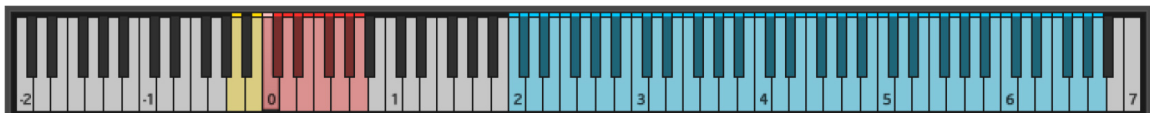
The Kontakt on-screen keyboard displaying the active keyswitches (in red), trigger keys (in blue), and solo keyswitches (in yellow)
