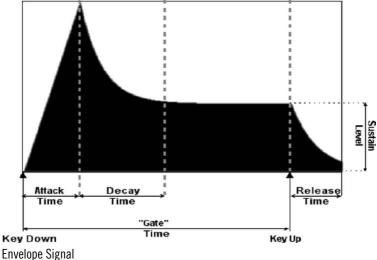
Modifying the Filter Envelope controls can provide a great range of effects on the output sound. Example Two in the the chapter "Exploring Patches" (Brass Ensemble on page 40) provides a few examples of the flexibility of the Filter Envelope.
