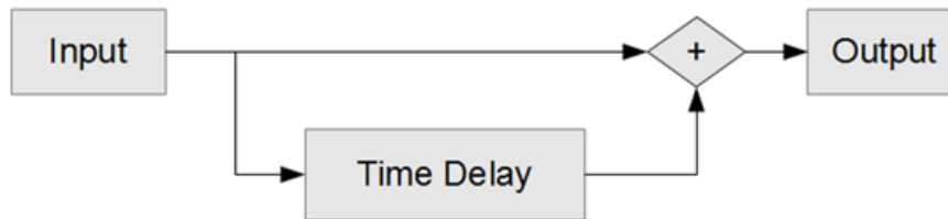
The Signal Flow Diagram of a Basic Echo Effect
