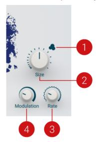
(1) **Density**: Switches between two basic density modes for the the reverb effect, Sparse and Dense. Sparse produces a dispersed, direct reverb sound. Dense produces a more washed-out, uniform reverb sound.
