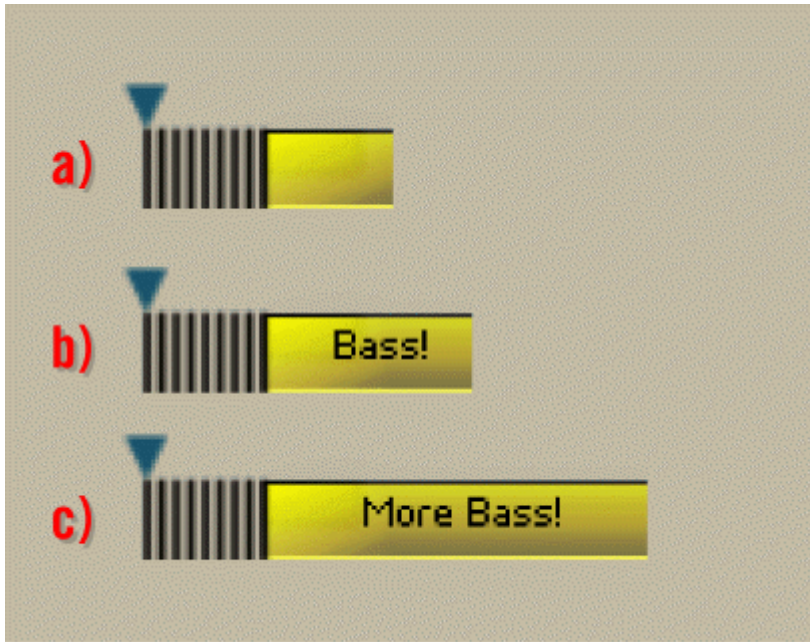
Fig. 8.23 Using the Border Left edit field in the Picture Properties dialog, the original skin in a) is resized to include a longer text fields on the right for b) and c).
