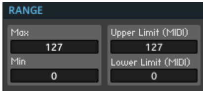
Fig. 9.31 The “Min”, “Max”, “Lower Limit”, and “Upper Limit” values can be set in the corresponding edit fields of the MIDI Source Module's Function page.
