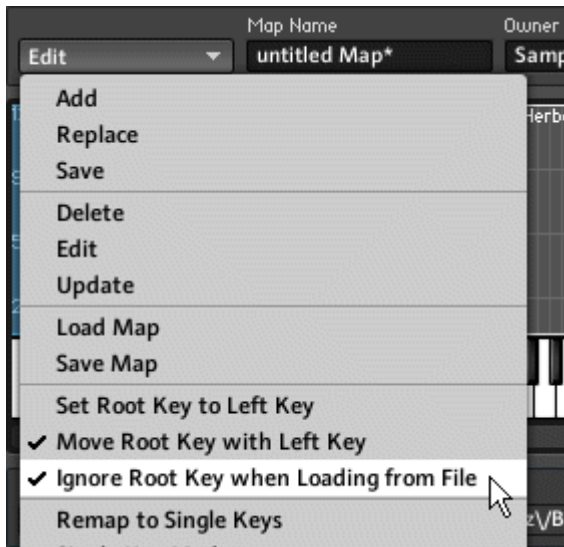
Fig. 6.15 To ignore any information tied to the Root value when loading a sample, choose the Ignore Root Key when Loading from File menu entry.
