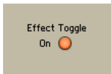
Fig. 8.7 With the 1 Toggle Button checkbox engaged, the Buttons Panel representation of a Switch Module becomes just one toggle button.
