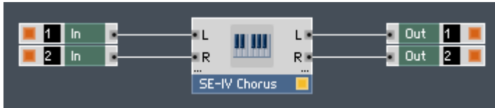
Fig. 7.27 You can use REAKTOR as an effect unit by using the signal from the Audio In Module as the dry signal for your effect Instrument and then routing the output of the effect to the input ports of the Audio Out Module.
