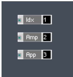
Fig. 12.3 When sending a value from an amplitude control to the Sine Bank Module, you need the index value, amplitude value, followed by an “apply” Event (in that particular order). For each new amplitude value, these three Events are sent from the “Idx”, “Amp”, and “App” output ports of the Macro, respectively.
