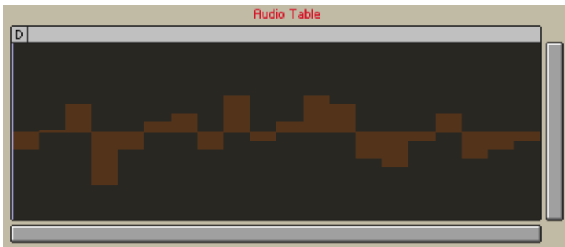
Fig. 11.5 The Fill graph style causes the area between the values and the x-axis to be filled with color. It is the Line + Fill graph style without the lines.
