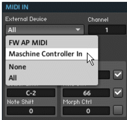
Fig. 13.2 With the External Device drop-down menu you can choose which MIDI device your Instrument should receive MIDI messages from. Note the entries “None” and “All”.
