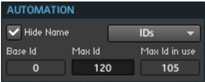
Fig. 14.13 The Base Id and Max Id in use displays as well as the Max Id edit field are found in the Automation area of the Instrument's Connections page. These fields give you information about the organization of the Instrument's list of Automation IDs.
