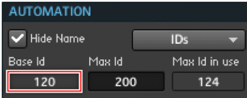
Fig. 14.14 The Base Id of the second Instrument is equal to the sum Base Id and Max Id of the previous Instrument.
