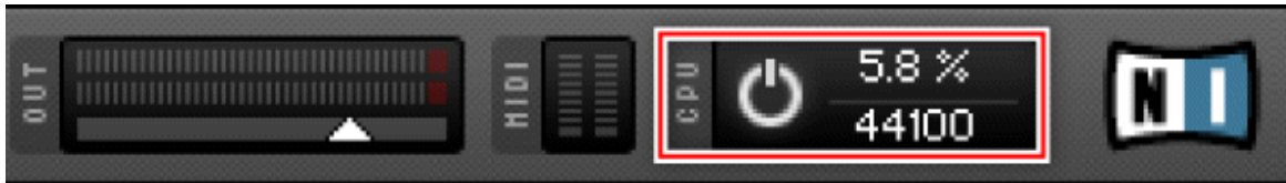
Fig. 3.64 The CPU area holds the Audio Engine button, the CPU Meter, and the Sample Rate drop-down menu.
