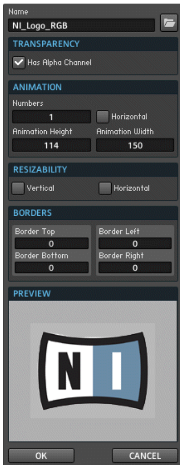
Fig. 8.19 You can make certain areas of a Targa picture file transparent by the use of an alpha channel. On REAKTOR's side, the Has Alpha Channel checkbox has to be engaged in order for the alpha channel to be recognized.
