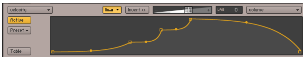
The curve editor allows you to create continuous, smooth modulation shapes.
