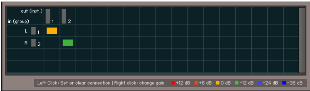
A routing configuration which keeps the channel order and assignment intact, but lowers the second channel by -12 dB in volume.
