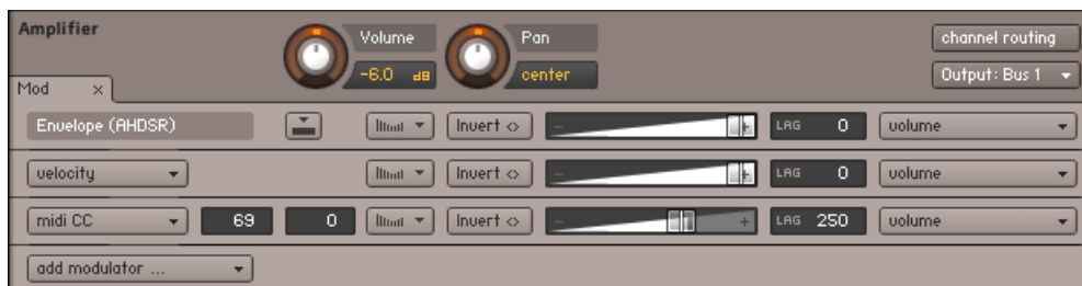
The Modulation Router of an Amplifier Module
