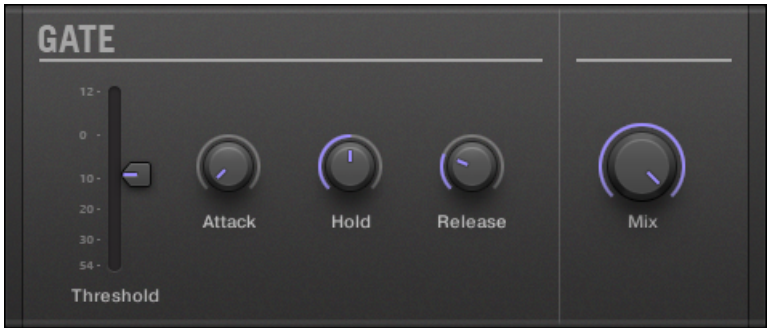
The Gate panel in the Plug-in Strip.
