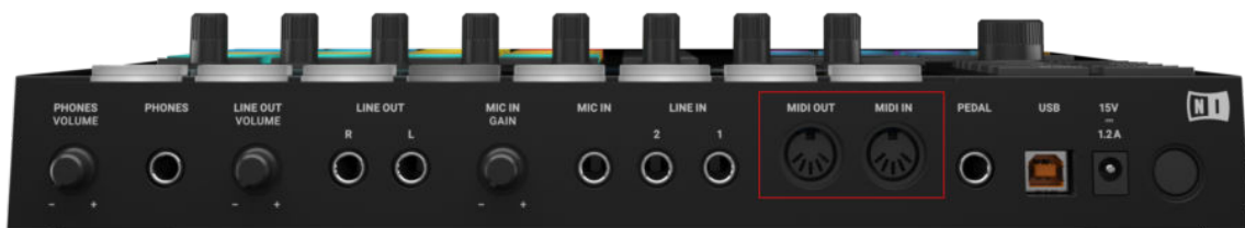
The MIDI sockets on the rear panel of the Maschine controller.
