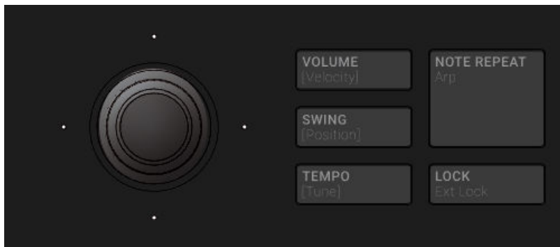
The Encoder situated to the left of the VOLUME , SWING and TEMPO buttons.
