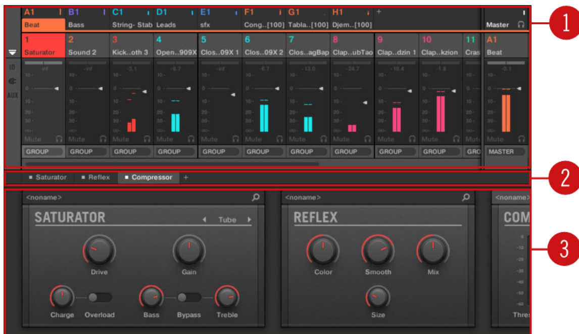
The Mix view, with the Mixer (1) at the top, the Plug-in Chain (2) in the middle, and the Plug-in Strip (3) at the bottom.
