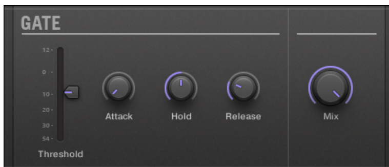
The Gate panel in the Plug-in Strip.
