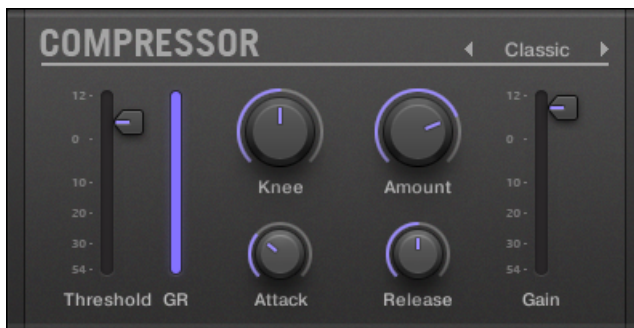
The Compressor panel in the Plug-in Strip.
