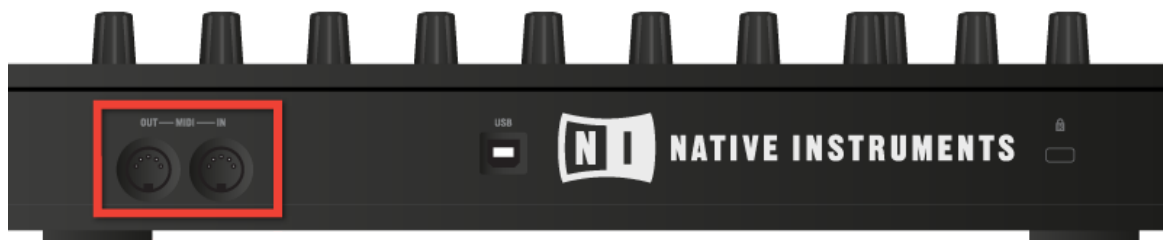
The rear side of the MASCHINE hardware with the MIDI IN and OUT sockets.
