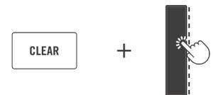
While holding MACRO, LEVEL, AUX, CONTROL, TUNE or SWING, double tap on a Smart Strip to reset the parameter to default.
