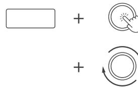
Step Modulation and Quick Edit can be used for both Step and Piano Roll mode. You can edit several notes or steps at the same time by pressing and holding them.
