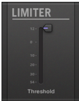
The Limiter panel in the Plug-in Strip.
