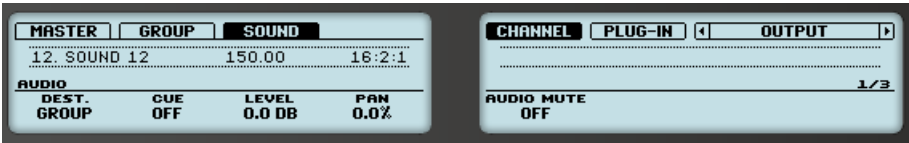
The AUDIO page of the Output properties (here for a Sound) on the controller.
