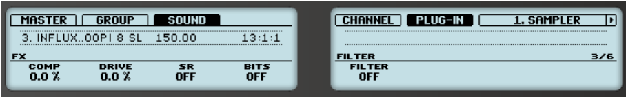
Sampler parameters – page 3 of 6: FX and FILTER on the controller.
