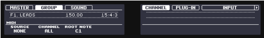
The MIDI page of the Input properties (here for a Group) on the controller.
