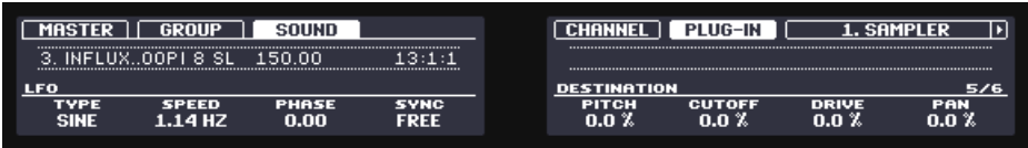
Sampler parameters – page 5 of 6: LFO and DESTINATION on the controller.
