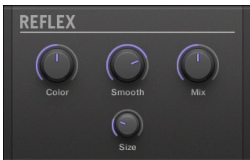
The Reflex panel in the Plug-in Strip.
