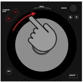
2. To slightly slow down the track's tempo, touch the outer rim of the Jog Wheel and turn it counterclockwise. Simultaneously, move the **TEMPO** fader slightly up.
