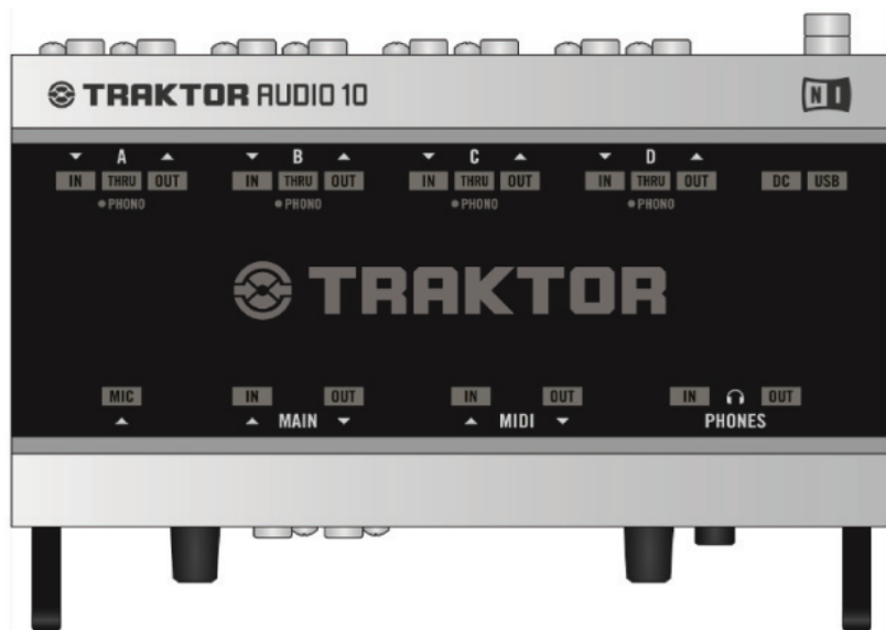
5.3 The top panel on the TRAKTOR AUDIO 10
