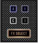
2. Press one of the dimly lit Deck Assign buttons B or D to switch to the right Deck side. These buttons will light brightly.
