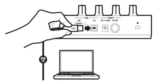
2. Connect the computer end (flat rectangle plug) of the USB cable to an available USB 2.0 port (or later) on your computer.
