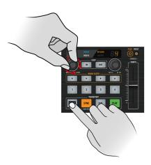
Holding SHIFT + turning the MOVE encoder to adjust TRAKTOR DJ's viewing scale.
