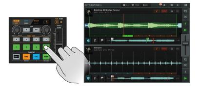
Triggering HotCue button 4 in TRAKTOR DJ's Loop Slicer mode.
