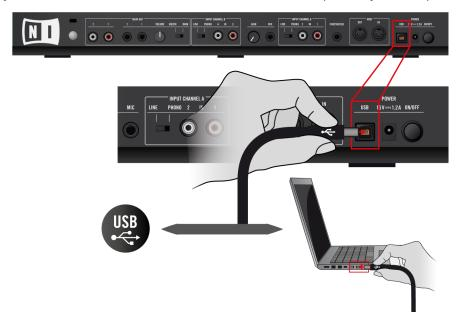
The TRAKTOR KONTROL S4 is a USB 2.0 device and will not work on a USB 1.0/1.1 port.
