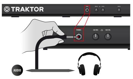
Before putting on headphones, always make sure the headphone volume knob (CUE VOL) is set to minimum! To set the headphone volume to minimum, turn the CUE VOL knob counterclockwise until it reaches its end stop. Then, while playing music, slowly increase the headphone volume by turning the CUE VOL knob clockwise until it reaches the desired listening level.
