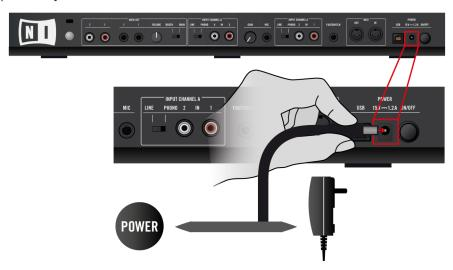
We strongly recommend you to use an external power supply with your S4 via the included power supply unit. Although operation is also possible when your S4 is powered via the USB connection, you then have following limitations: the headphones output level is lower, and all LEDs light darker. Moreover, your device might then be subject to USB power-related issues, as explained in section \$\gamma 9.2.4\$, USB-related Power Issues.
