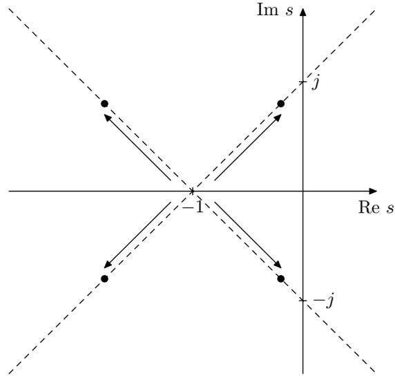
Figure 5.2: Poles of the 4-pole lowpass ladder filter.
