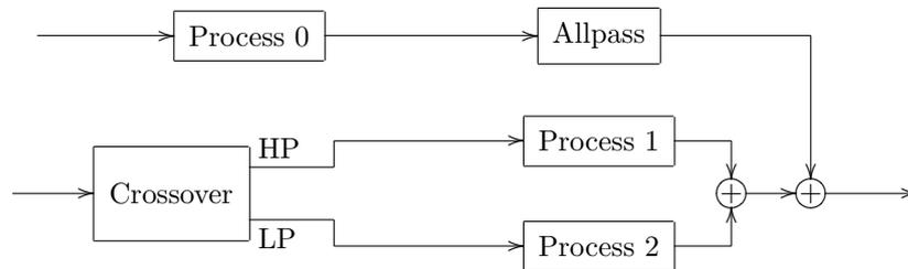
Figure 10.20: Correction allpass at the end of processing.
