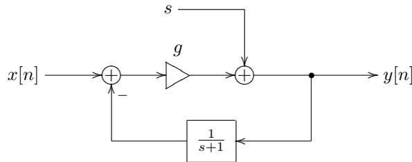
Figure 3.36: An instantaneous representation of a digital 1-pole lowpass filter with a trapezoidal integrator and an analog lowpass smoother.
