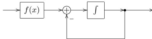
Figure 6.66: Waveshaper followed by a 1-pole lowpass.
