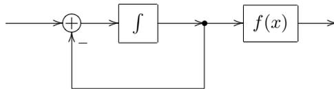
Figure 6.74: 1-pole lowpass followed by a waveshaper.
