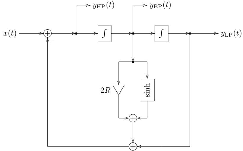
Figure 6.51: A second attempt to introduce an antisaturator into an SVF (works better, but  $R$  does no longer correspond to damping).
