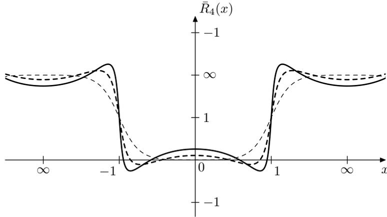
Figure 9.60: Normalized elliptic rational function for  $k = 0.9$  (solid),  $k = 0.7$  (dashed) and  $k = 0$  (thin dashed).
