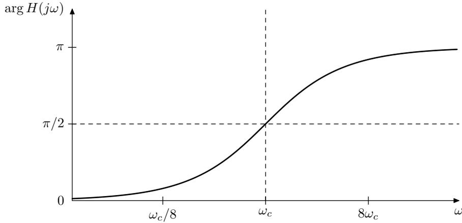
Figure 10.37: Phase response of a negative-cutoff 1-pole allpass filter.
