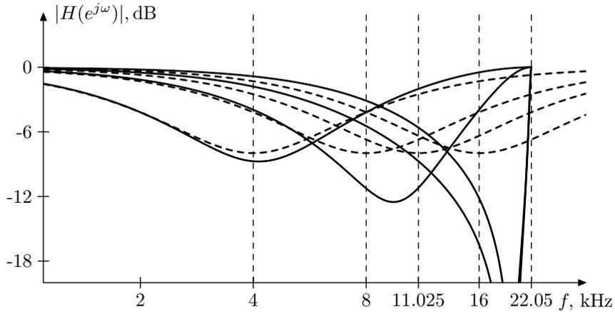
Figure 3.25: Separate prewarping of system components (for a number of different cutoffs). Dashed curves represent the respective analog filter responses for the same cutoffs. Sampling rate 44.1kHz.
