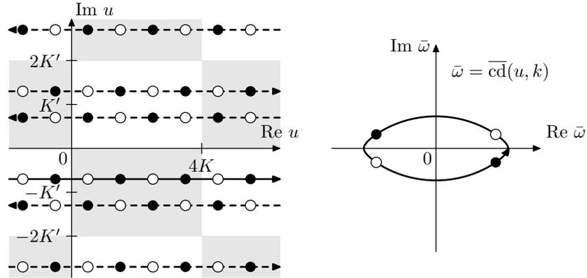
Figure 9.64: Transformation of Fig. 9.63 by  $u = Kv/N\tilde{K}$  (for  $N = 2$ ). The white and black dots on the quasielliptic curve are even/odd elliptic poles in terms of  $\bar{\omega}$ . (The picture is qualitative.)
