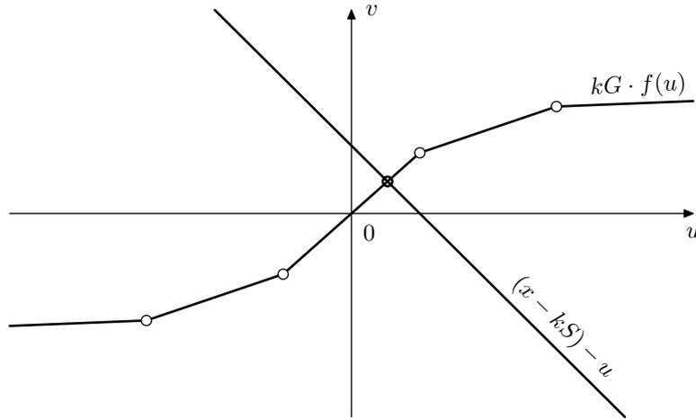
Figure 6.28: The solution of (6.13) for a piecewise-linear saturator.
