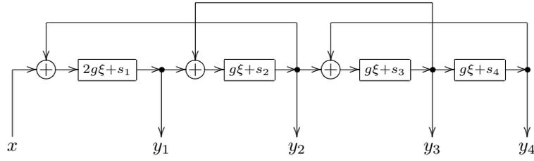
Figure 5.52: Diode ladder in the instantaneous response form.
