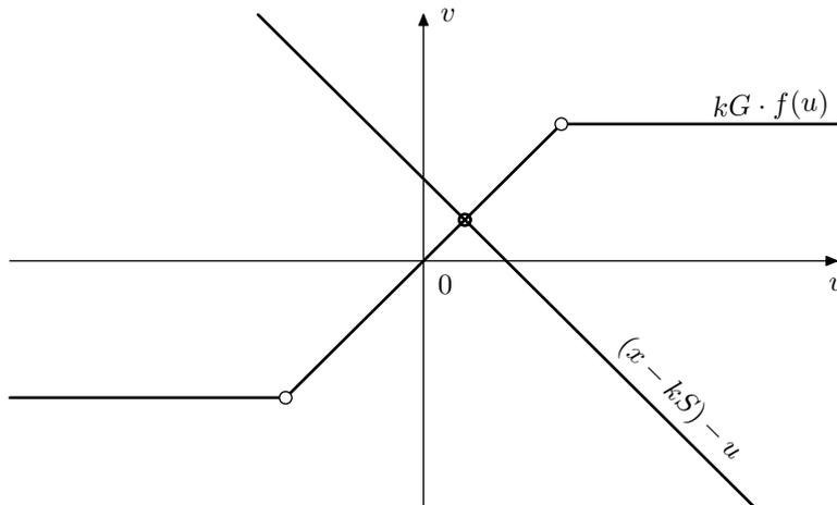
Figure 6.29: The solution of (6.13) for a hard clipper.
