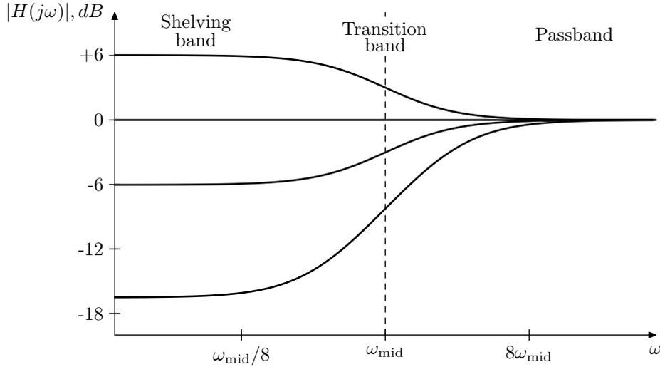
Figure 10.4: Amplitude responses of a 1-pole low-shelving filter.
