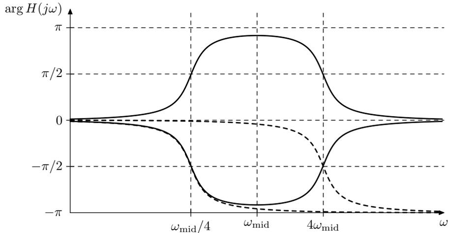
Figure 10.10: Phase response of the 2-pole tilting filter for  $M = 4$  (positive) and for  $M = 1/4$  (negative). Damping  $R = 1/4$ . Dashed curves represent phase responses of the underlying 2-pole lowpasses at cutoffs  $M$  and  $M^{-1}$ .
