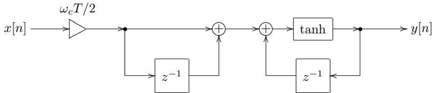
Figure 6.39: Saturating direct form I trapezoidal integrator.
