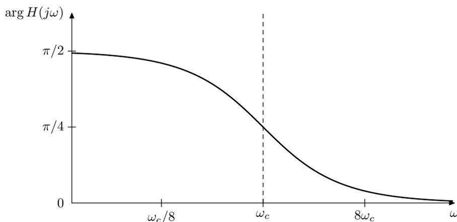
Figure 2.11: Phase response of a 1-pole highpass filter.
