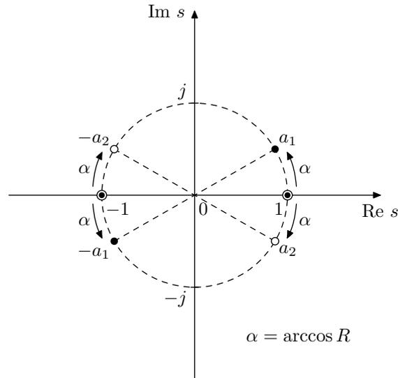
Figure 8.20: Roots of  $Q(s)$  for  $0 < R < 1$  (black dots are roots of  $Q_1(s)$ , white dots are roots of  $Q_2(s)$ ) and their positions at  $R = 1$  (indicated by circled dots, where each such dot denotes a root of  $Q_1(s)$  coinciding with a root of  $Q_2(s)$ ).
