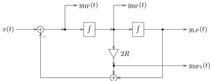
Figure 4.17: State-variable filter with a normalized bandpass output.
