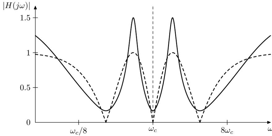
Figure 11.12: Amplitude response of the mult notch in Fig. 11.11 built around a chain of 6 identical 1-pole allpasses at  $k = 0.5$ . Dashed curve corresponds to  $k = 0$  (the same response as in Fig. 11.4).
