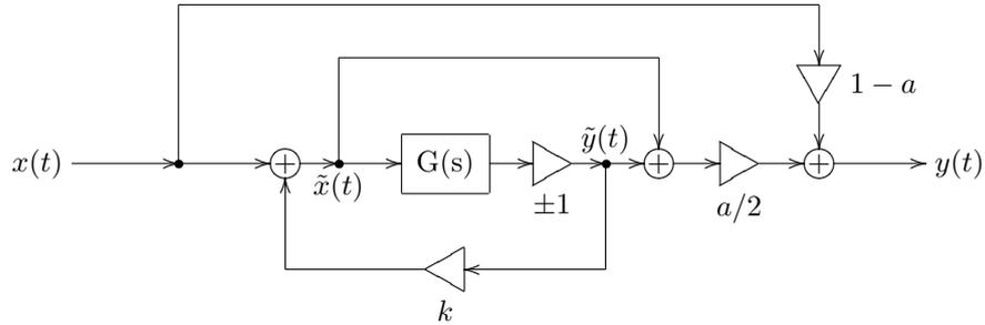
Figure 11.17: Multinotch with feedback, inversion and dry/wet mixing.
