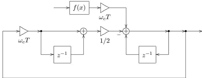
Figure 6.73: Structure from Fig. 6.67 with the waveshaped signal bypassing the first part of the direct form I integrator (thereby compensating the introduced latency) but without repositioning of  $\omega_cT$  gain element.
