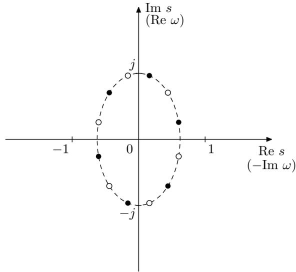
Figure 9.26: Chebyshev type I filter's even (white) and odd (black) poles for  $N = 6$  (including the poles of  $H(-s)$ ).
