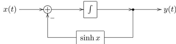
Figure 6.49: Lowpass filter's state saturation by using an antisaturator.
