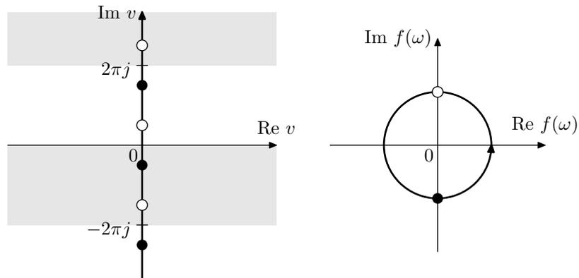
Figure 9.13:  $f(\omega)$  moving in a unit-radius circular trajectory, the points  $f(\omega) = \pm j$  and their preimages.
