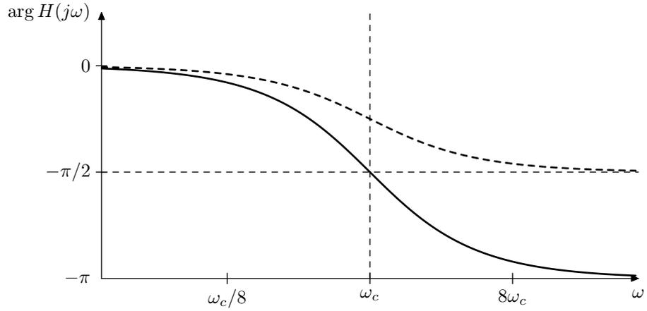
Figure 4.12: Phase response of the 2-pole lowpass filter at  $R = 1$  (solid line) compared to the amplitude response of the 1-pole lowpass filter (dashed line).
