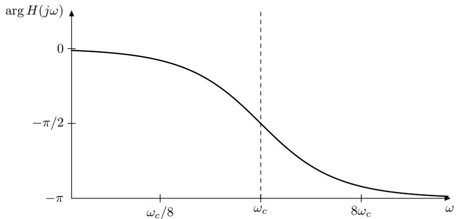
Figure 2.18: Phase response of the 1-pole allpass filter (2.12).
