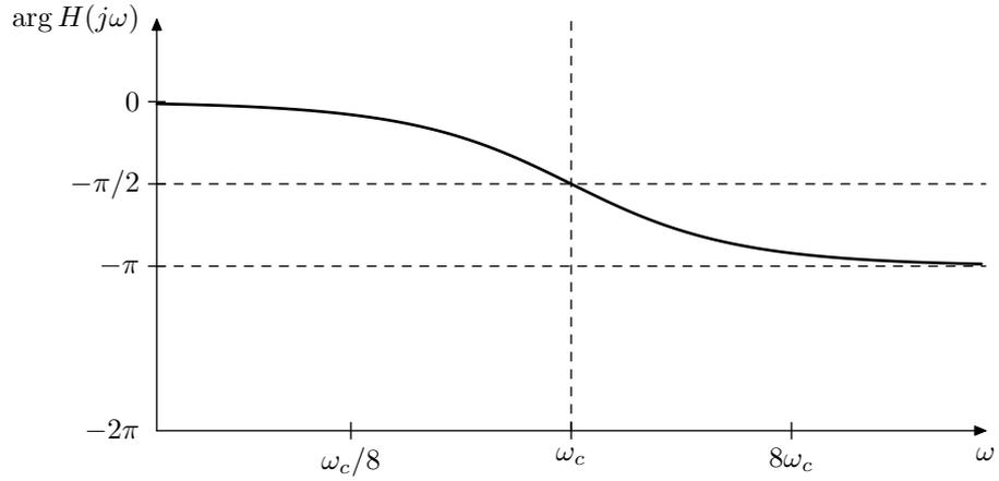
Figure 10.35: Phase response of a 1-pole allpass filter.
