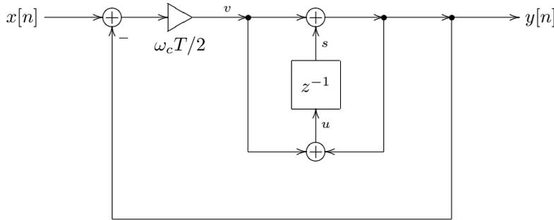
Figure 3.30: 1-pole TPT lowpass filter with helper variables.
