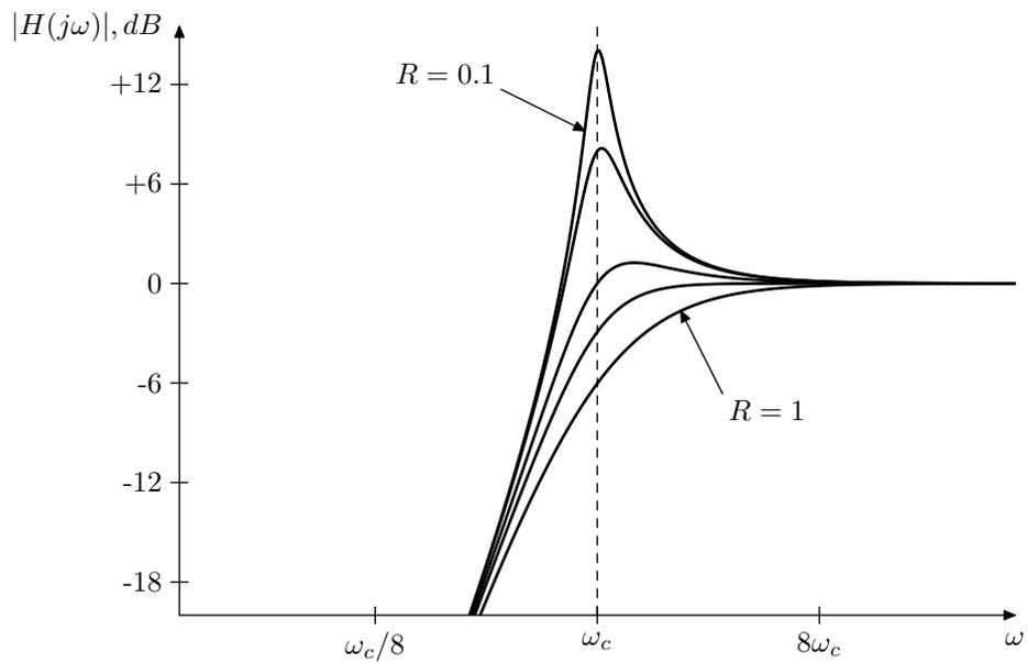
Figure 4.4: Amplitude response of a 2-pole highpass filter.
