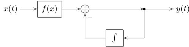
Figure 6.79: Waveshaper followed by a 1-pole highpass.
