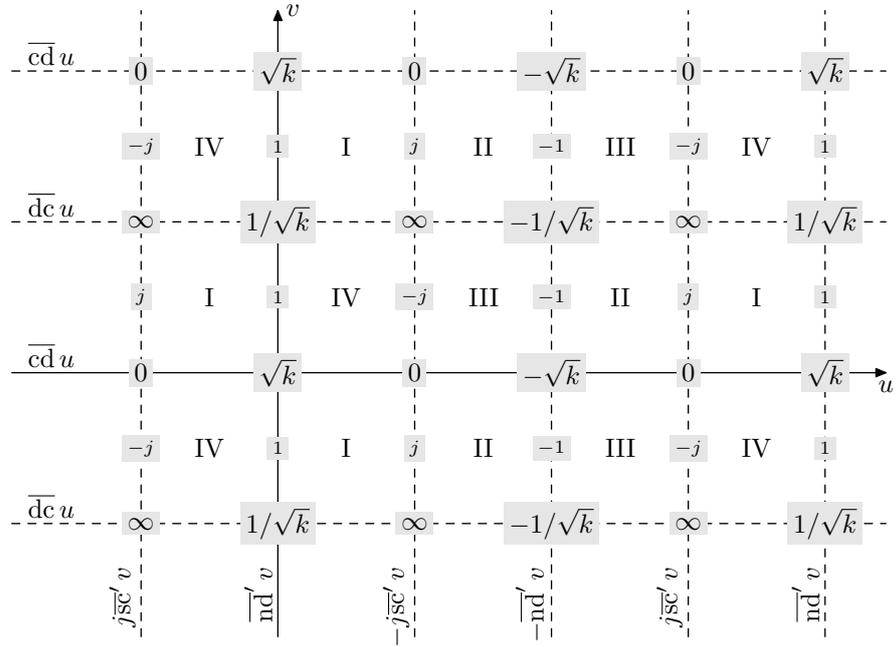
Figure 9.50: Values of  $\overline{cd} x = \overline{cd}(u + jv)$  on the quarter-period grid (compare to Fig. 9.42).
