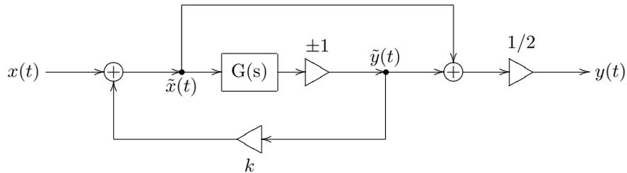
Figure 11.15: Mult notch with feedback and inversion.
