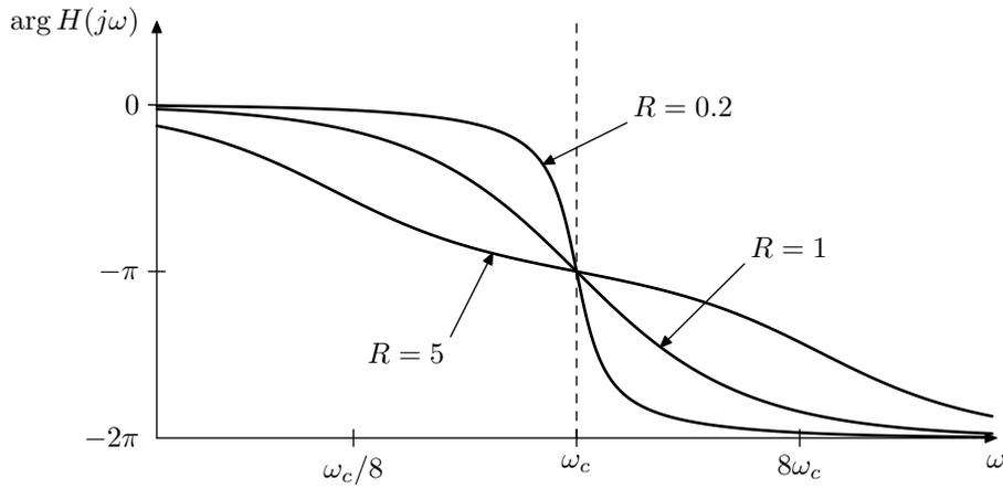
Figure 4.23: Phase response of a 2-pole allpass filter.
