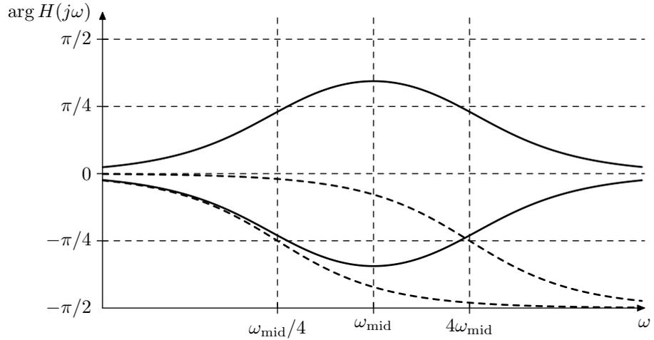
Figure 10.6: Phase response of the 1-pole shelving/tilting filters for  $M = 4$  (positive) and for  $M = 1/4$  (negative). Dashed curves represent phase responses of the underlying 1-pole lowpasses at cutoffs  $M$  and  $M^{-1}$ .
