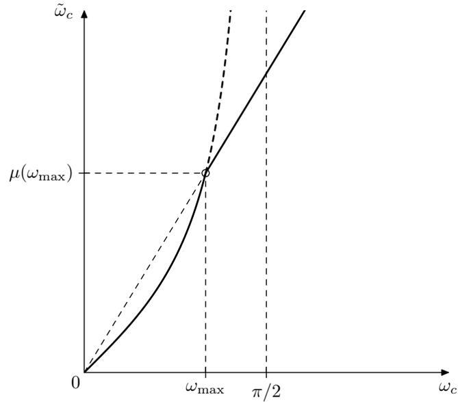
Figure 3.24: Bounded cutoff prewarping. The thick dashed line shows the unbounded prewarping continuation. The thin oblique dashed line is the continuation of the straight part of the prewarping curve. The black dot marks the breakpoint of the prewarping curve.
