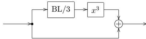
(where BL/3 denotes a filter which bandlimits the signal to 1/3 of the Nyquist frequency, and Lat denotes). Actually bandlimiting will introduce latency into the signal, so we'll need to add the same latency on the lower path
