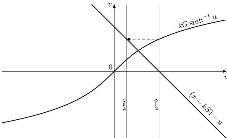
Figure 6.23: Initial bracketing for bisection in the case of an unbounded saturator and  $k \geq 0$ . First we find the right bracket  $b$  and then use  $v = kG \sinh^{-1} b$  to find the left bracket  $a$ .
