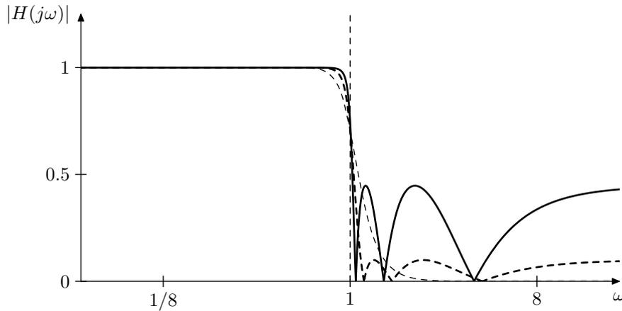
Figure 9.31: Chebyshev type II filter's amplitude responses for  $N = 6$  and  $\varepsilon = 0.5$  (solid),  $\varepsilon = 0.1$  (dashed) and  $\varepsilon = 0$  (Butterworth, thin dashed). Notice the usage of the linear amplitude scale, which is chosen in order to be able to show the amplitude response zeros.
