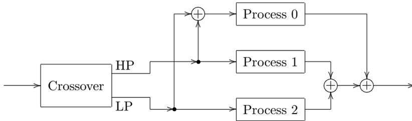
Figure 10.18: Adjusting the phase of the bypass signal.
