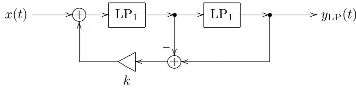
Figure 5.26: TSK filter (alternative representation, negative feedback form).
