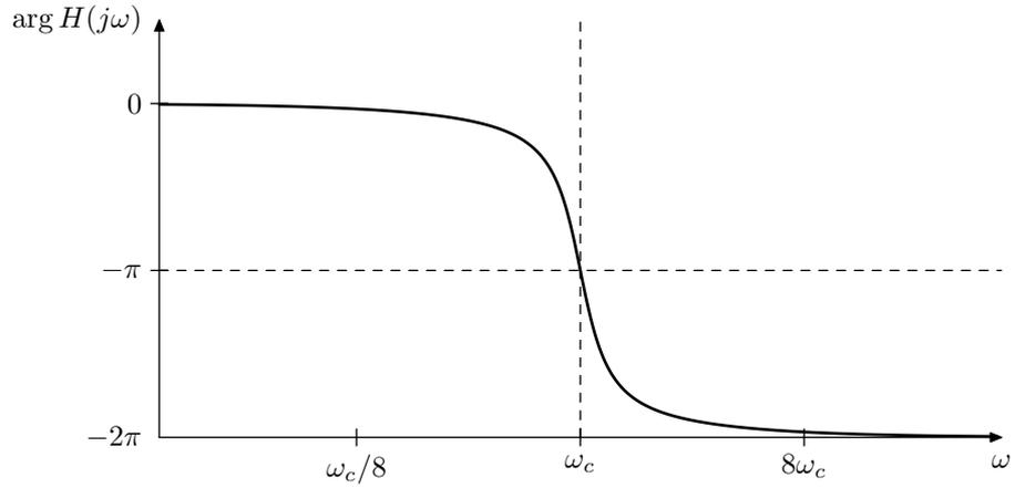
Figure 10.36: Phase response of a 2-pole allpass filter.
