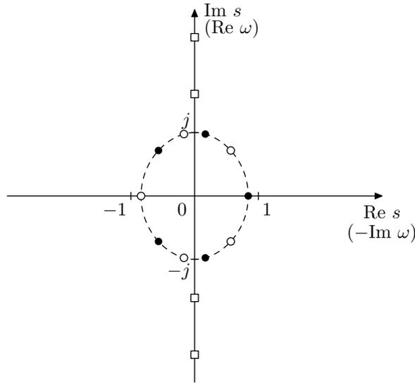
Figure 9.65: Poles (white and black dots) and zeros (white squares) of an elliptic filter of order  $N = 5$ . Each of the zeros is duplicated, but the duplicates are dropped together with the unstable poles.
