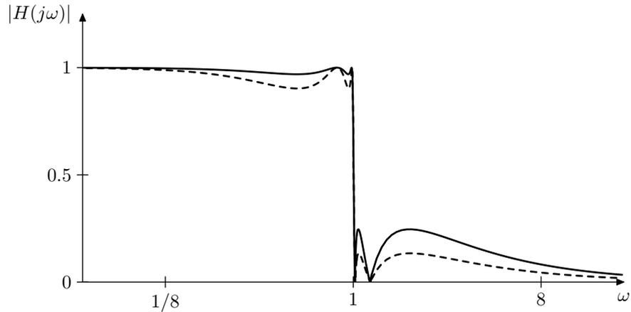
Figure 9.62: Elliptic filter's amplitude responses for  $N = 5$ ,  $k = 0.98$  and  $\lambda = 1$  (solid) and  $\lambda = k^{-1/4}$  (dashed). Notice the usage of the linear amplitude scale, which is chosen in order to be able to show the amplitude response zeros.
