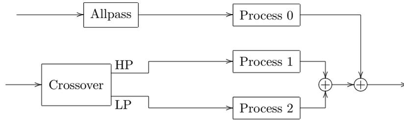
Figure 10.19: Adjusting the phase of the signal from a different source.
