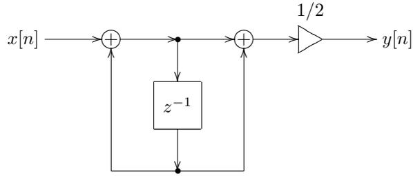
Figure 3.9: Direct form II (canonical) trapezoidal integrator ( $T = 1$ ).
