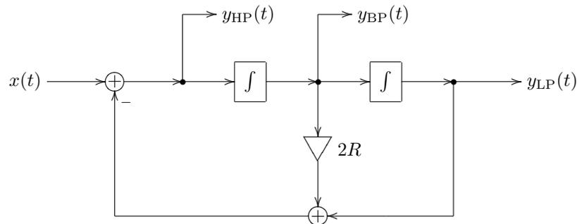
Figure 4.1: 2-pole multimode state-variable filter.
