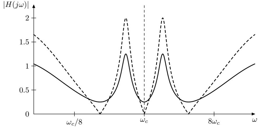
Figure 11.16: Amplitude response of the multinotch in Fig. 11.13 built around a chain of 6 identical 1-pole allpasses at  $k = 0.5$  with a dry/wet mixing ratio of 50%. Dashed curve corresponds to a dry/wet mixing ratio of 100% (same response as in Fig. 11.14).
