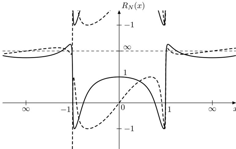
Figure 9.56: Elliptic rational functions of even (solid) and odd (dashed) orders for  $k = 0.99$ . The graphs do not cross the horizontal axis at  $x = 1$ , rather  $R_N(1) = 1 \forall N$ , however the resolution of the figure is insufficient to see that. The poles of  $R_N$  are occurring at the intersections of the respective graph with the thin horizontal dashed line at  $\infty$ .
