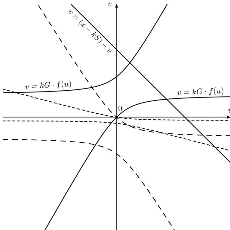
Figure 6.27: Choice of the solution of the quadratic equation for  $f(u)$  which is a member of the family of hyperbolas (6.24). Solid line corresponds to  $kG > 0$ , dashed lines correspond to two different values of  $kG < 0$ .
