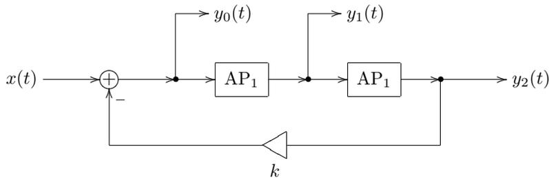
Figure 5.34: 2-pole ladder filter based on allpasses (not so useful).
