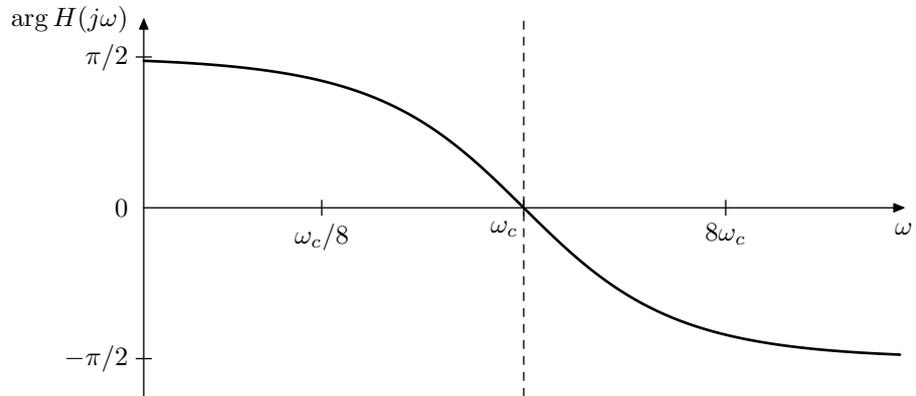
Figure 2.17: Phase response of the 1-pole allpass filter (2.11).
