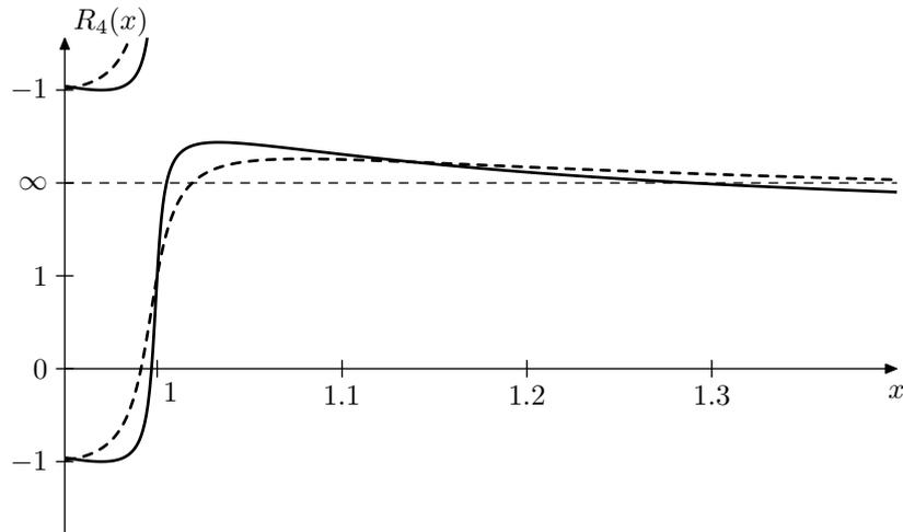
Figure 9.57: Transition region of  $R_4(x)$  for  $k = 0.998$  (solid) and  $k = 0.99$  (dashed). The horizontal axis is linear, the vertical axis is using the arctangent scale.
