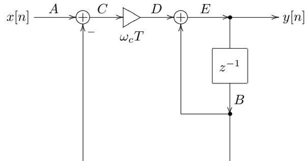
Figure 3.27: Naive 1-pole lowpass filter and the respective signal computation order.
