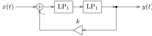
Figure 5.20: 2-pole lowpass ladder filter (not very useful).
