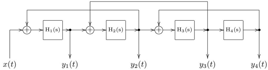
Figure 5.50: Generalized diode ladder in transfer function form.
