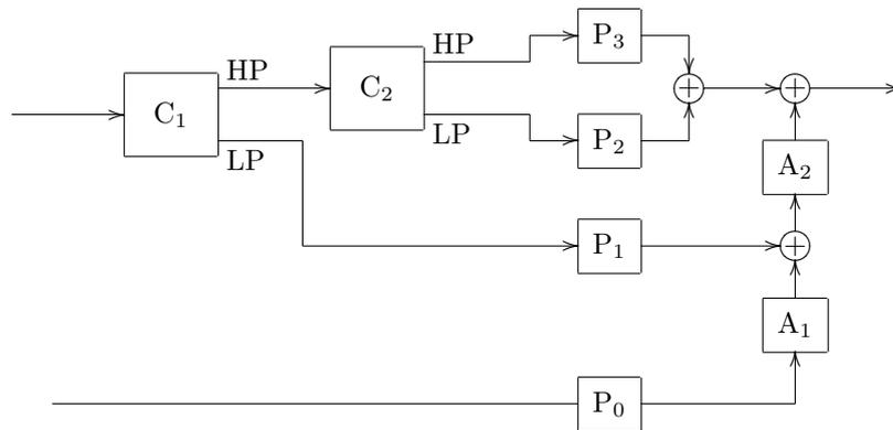
Figure 10.24: 3-way crossover mixing with all phase correction done at the end.
