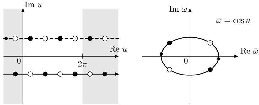
Figure 9.25: Transformation of Fig. 9.24 by  $u = v/N$  (for  $N = 2$ ). The white and black dots on the ellipse are even/odd Chebyshev poles in terms of  $\bar{\omega}$ . (The picture is qualitative, as the scales of the real and imaginary axes in the  $u$  plane are not equal.)
