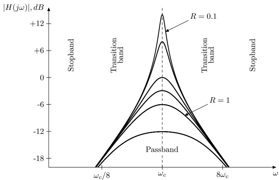
Figure 4.5: Amplitude response of a 2-pole bandpass filter.
