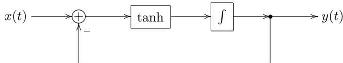
Figure 6.35: OTA-style nonlinear 1-pole lowpass.
