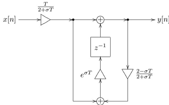
Figure 3.39: Transposed direct form II-style “unstable” trapezoidal integrator.
