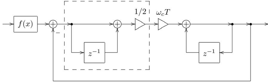
Figure 6.68: Structure from Fig. 6.67 with a changed position of the cutoff gain.
