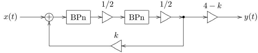
Figure 5.18: 4-pole normalized bandpass ladder filter expressed in terms of normalized 2-pole bandpasses.
