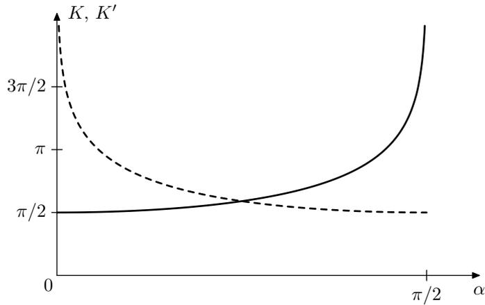
Figure 9.34: Complete elliptic integral of the first kind  $K$  (solid line) and the complementary complete elliptic integral of the first kind  $K'$  (dashed line), plotted against the modular angle  $\alpha$ .
