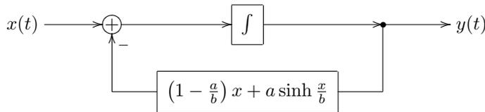
Figure 6.48: Diode clipper with cutoff-independent leakage (simplified diagram).
