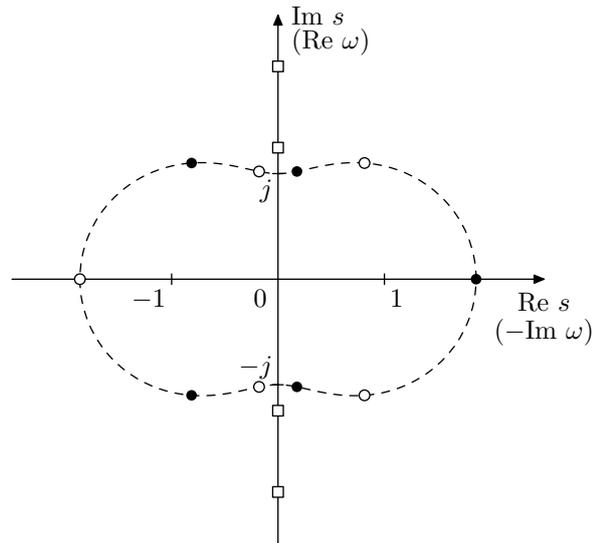
Figure 9.32: Poles (white and black dots) and zeros (white squares) of a Chebyshev type II filter of order  $N = 5$ . Each of the zeros is duplicated, but the duplicates are dropped together with the unstable poles.
