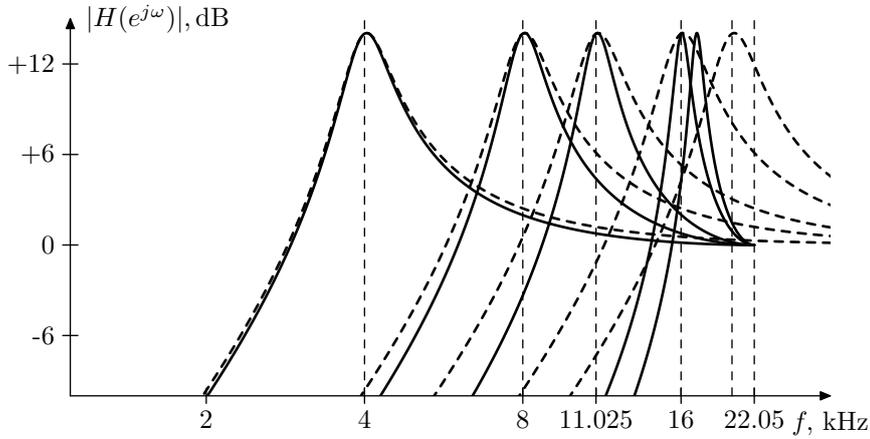
Figure 3.22: Effect of cutoff prewarping bounded at 16kHz. Sampling rate 44.1kHz.
