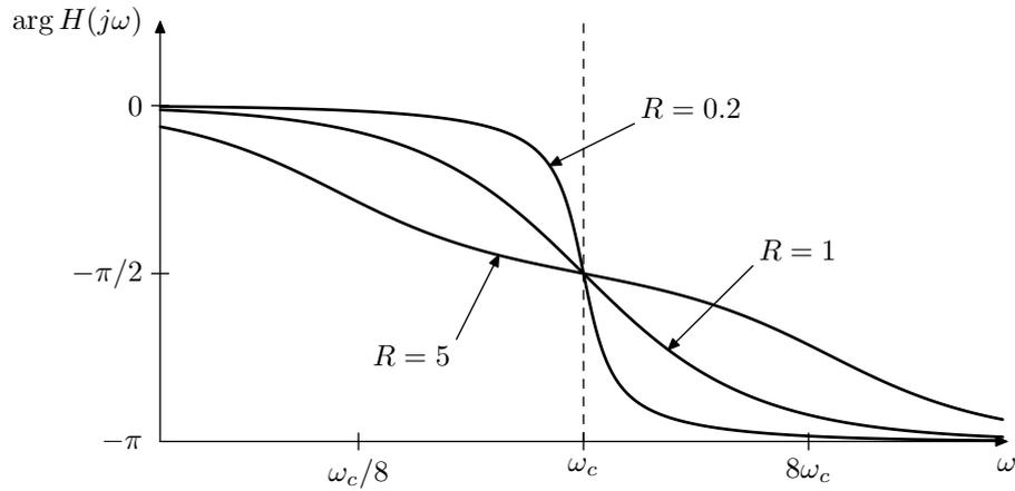
Figure 4.6: Phase response of a 2-pole lowpass filter. Bandpass and highpass responses are the same, except that they are shifted by  $+90^\circ$  and  $180^\circ$  respectively.
