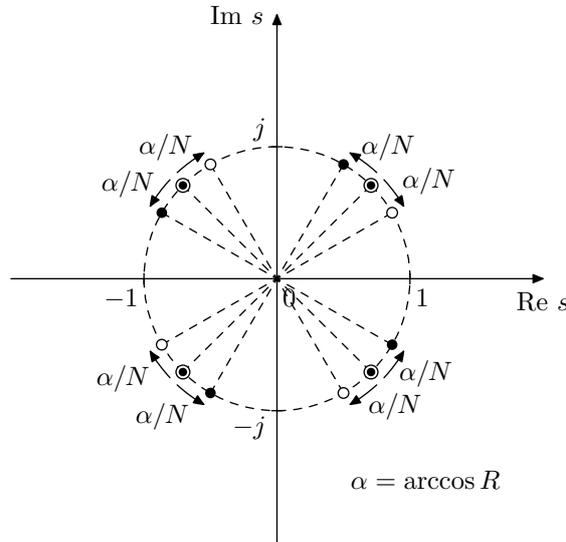
Figure 8.21: Roots of  $Q'(s)$  for  $0 < R < 1$  (black dots are roots of  $Q'_1(s)$ , white dots are roots of  $Q'_2(s)$ ) and their positions at  $R = 1$  (indicated by circled dots, where each such dot denotes a root of  $Q'_1(s)$  coinciding with a root of  $Q'_2(s)$ ). Butterworth transformation order  $N = 2$ .
