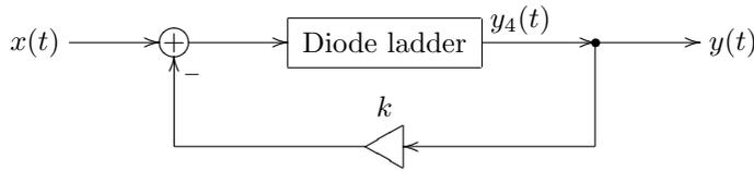
Figure 5.49: Diode ladder filter.
