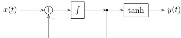
Figure 6.37: Putting a saturator at the filter's output.
