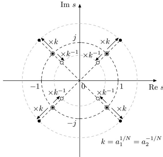
Figure 8.19: Roots of  $Q'(s)$  for  $R > 1$  (black dots are roots of  $Q'_1(s)$ , white dots are roots of  $Q'_2(s)$ ) and their positions at  $R = 1$  (indicated by circled dots, where each such dot denotes a root of  $Q'_1(s)$  coinciding with a root of  $Q'_2(s)$ ). Butterworth transformation order  $N = 2$ .
