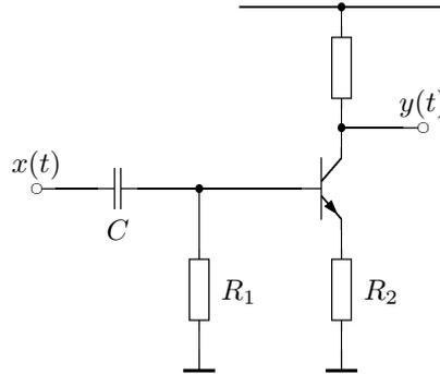
Figure 6.60: Highpass filter with asymmetric cutoff.
