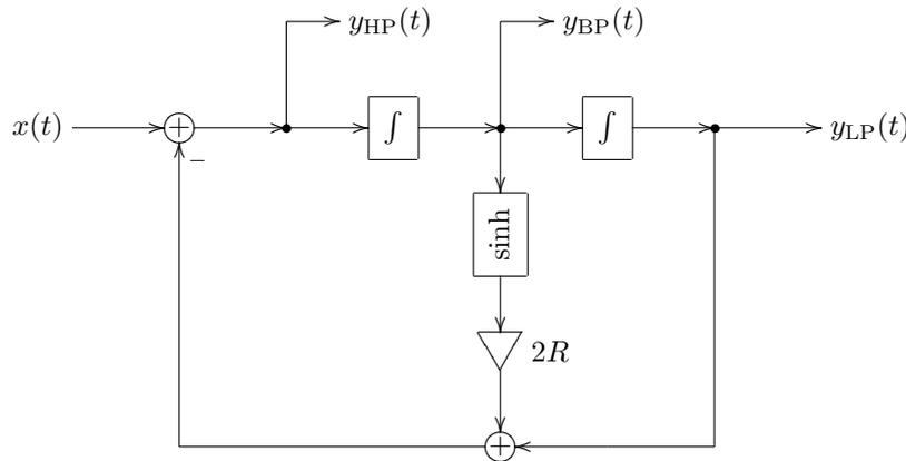
Figure 6.50: An attempt to introduce an antisaturator into an SVF (not really working).
