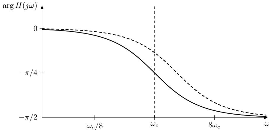
Figure 2.7: 1-pole lowpass filter's phase response shift by a cutoff change.
