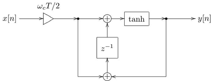
Figure 6.40: Saturating transposed direct form II trapezoidal integrator.
