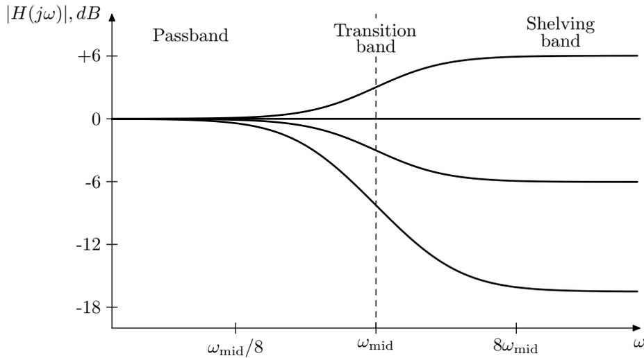
Figure 10.5: Amplitude responses of a 1-pole high-shelving filter.
