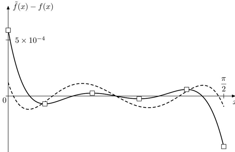
Figure 10.33: The error of the 4-th order polynomial approximations of  $\sin x$  on  $[0, \pi/2]$ . The approximation with uniformly spaced zeros at  $9^\circ, 27^\circ, 45^\circ, 63^\circ, 81^\circ$  (solid line) and the one with Chebyshev zeros (dashed line). The empty square-shaped dots at the extrema of the error are the control points of the Remez algorithm.
