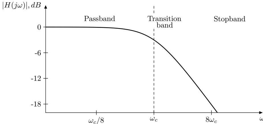
Figure 2.4: Amplitude response of a 1-pole lowpass filter.
