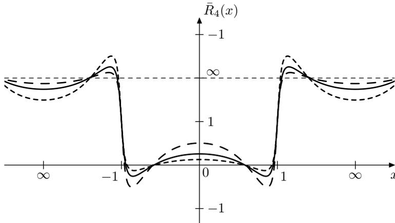
Figure 9.59: Renormalized elliptic rational function for  $\lambda = 1$  (solid),  $\lambda = k^{1/4}$  (small dashes) and  $\lambda = k^{-1/4}$  (large dashes). As the used elliptic modulus  $k = 0.9$  is pretty close to 1, the corresponding variations of the transition band width are not well visible.
