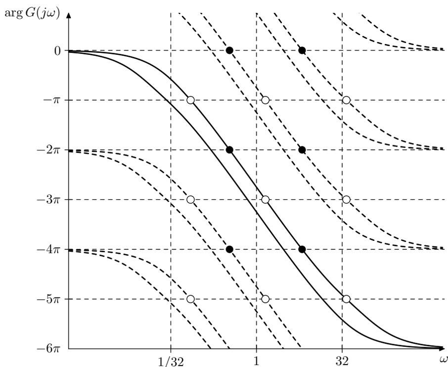
Figure 11.19: Phase responses of  $H_+^{-1}$  and  $H_-$  (each consisting of six 1-pole allpasses). The frequency shifter bandwidth is 10 octaves (bounded by vertical dashed lines at  $\omega = 1/32$  and  $\omega = 32$ ). Black dots correspond to multinotch's peaks arising out of  $H_+^{-1}$ , white dots correspond to the respective notches. Dashed curves show "aliased" phase responses.
