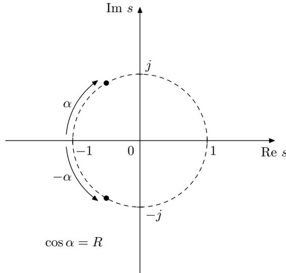
Figure 4.8: Poles of a resonating 2-pole filter ( $\omega_c = 1$ ).
