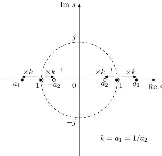
Figure 8.18: Roots of  $Q(s)$  for  $R > 1$  (black dots are roots of  $Q_1(s)$ , white dots are roots of  $Q_2(s)$ ) and their positions at  $R = 1$  (indicated by circled dots, where each such dot denotes a root of  $Q_1(s)$  coinciding with a root of  $Q_2(s)$ ).
