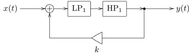
Figure 5.21: 2-pole bandpass ladder filter.
