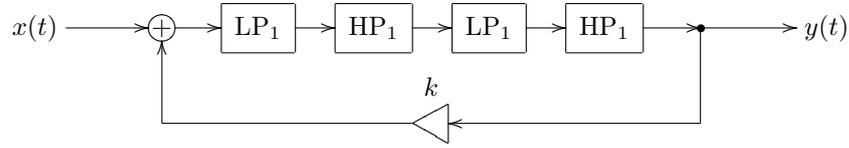
Figure 5.14: A “true” bandpass ladder filter.
