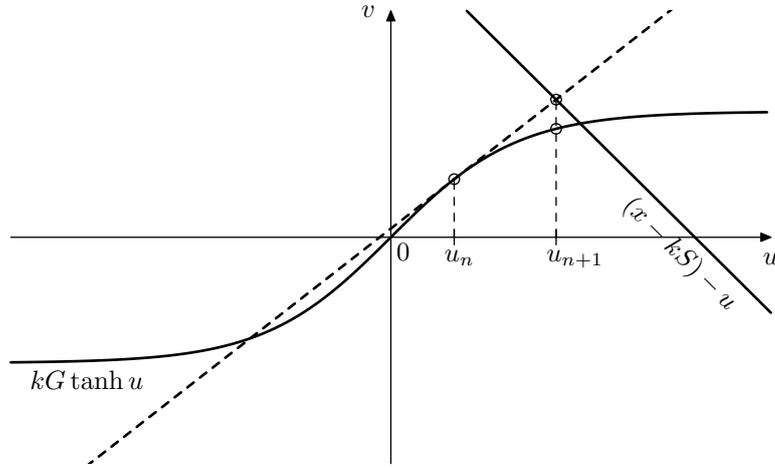
Figure 6.19: Newton–Raphson method: linearization by the tangent line.
