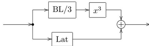
(where Lat denotes a structure which artificially introduces the same latency as introduced by BL/3).
