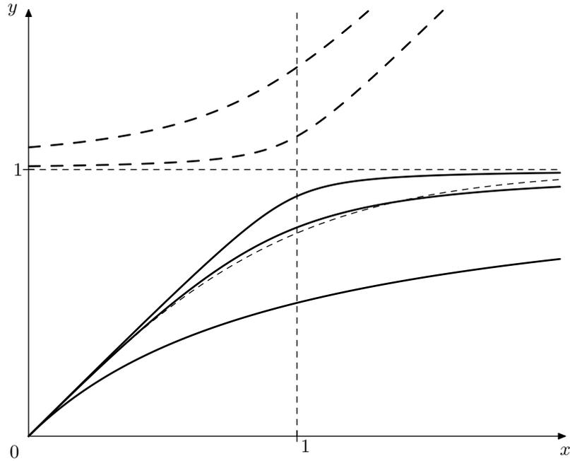
Figure 6.26: A family of soft clippers generated by (6.24) for  $y_1 = 0.5$ ,  $y_1 = 0.7829$  and  $y_1 = 0.9$ . The two dashed curves above the line  $y = 1$  are the second (unused) branches of the respective curves (the second branch for  $y_1 = 0.5$  is not visible because it is outside the picture boundaries). The thin dashed curve close to the main branch of the curve for  $y_1 = 0.7829$  is the hyperbolic tangent  $y = \tanh x$ .
