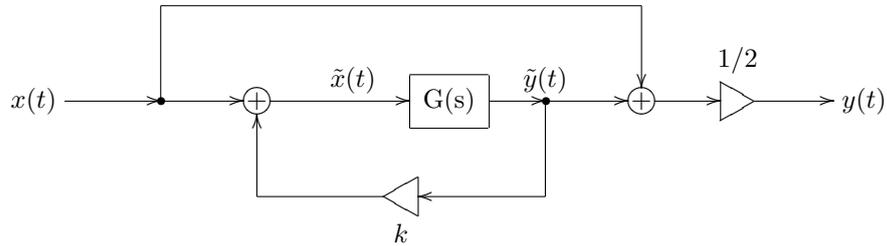
Figure 11.11: Multinotch from Fig. 11.1 with added feedback. Note that this figure is showing a poor mixing option.
