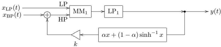
Figure 6.10: Sallen-Key filter with an asymptotically linear saturator.
