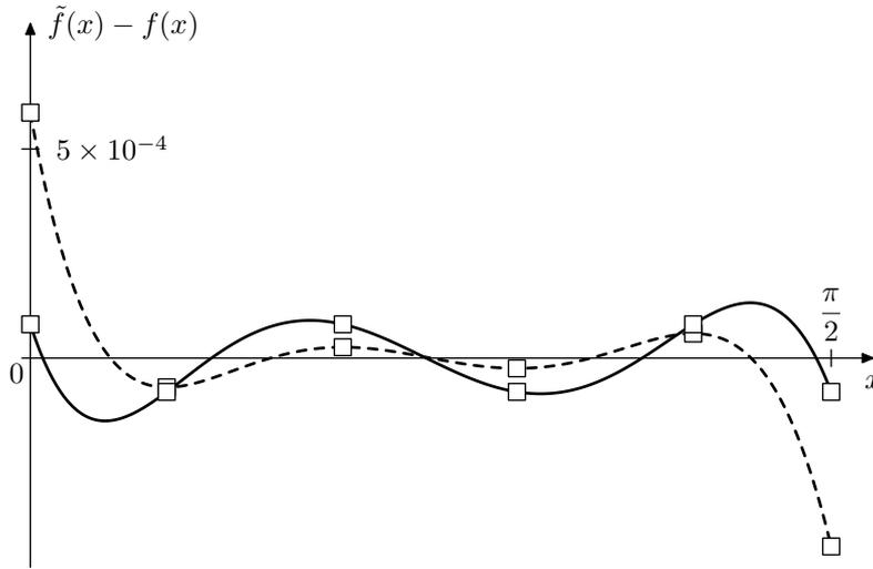
Figure 10.34: The approximation error before (dashed line) and after (solid line) a single step of the Remez polynomial approximation algorithm. The empty square-shaped dots are the control points.
