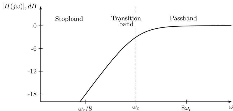
Figure 2.10: Amplitude response of a 1-pole highpass filter.
