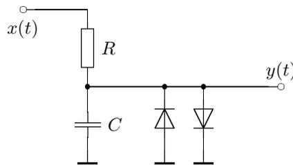
Figure 6.44: Diode clipper.
