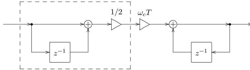
Figure 6.64: Structure in Fig. 6.63 implies positioning the  $\omega_c T$  gain element in the middle of the integrator. The dashed line highlights the part which is being replaced by the antialiased waveshaper.
