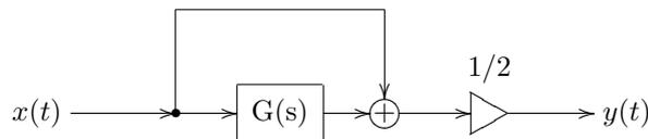
Figure 11.1: A basic multinotch.  $G(s)$  is an allpass.
