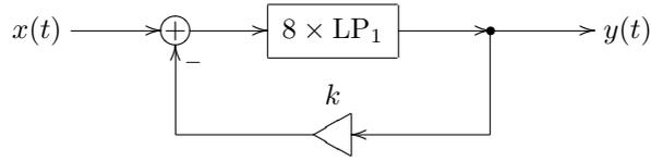
Figure 5.37: 8-pole lowpass ladder filter.
