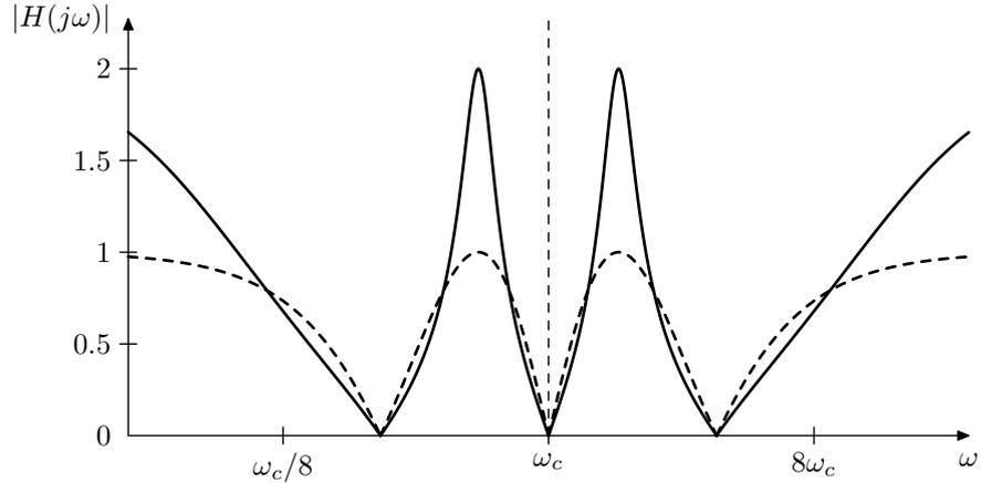
Figure 11.14: Amplitude response of the mult notch in Fig. 11.13 built around a chain of 6 identical 1-pole allpasses at  $k = 0.5$ . Dashed curve corresponds to  $k = 0$  (the same response as in Fig. 11.4).
