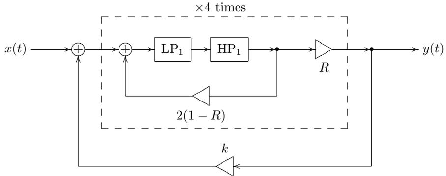
Figure 5.47: 8-pole bandpass ladder filter expressed in terms of halved normalized TSK bandpasses.
