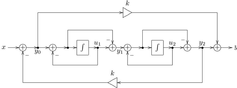
Figure 7.1: Allpass TSK filter from Fig. 5.35 with expanded 1-pole allpass structures.
