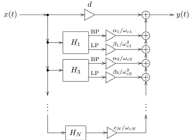
Figure 8.6: Implementation by parallel SVFs and 1-pole lowpasses.
