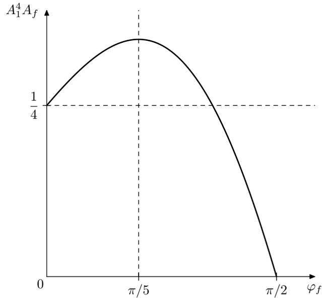
Figure 5.8: Total amplitude response of the four feedforward low-pass 1-poles plus the feedback lowpass 1-pole at the  $180^\circ$  phase shift point, plotted against the phase shift by the feedback 1-pole.
