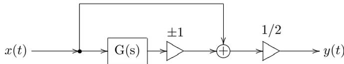
Figure 11.8: Multinotch from Fig. 11.1 with optional inversion.
