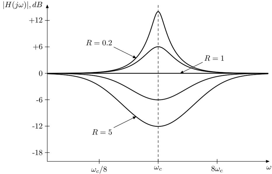
Figure 4.24: Amplitude response of a 2-pole peaking filter.
