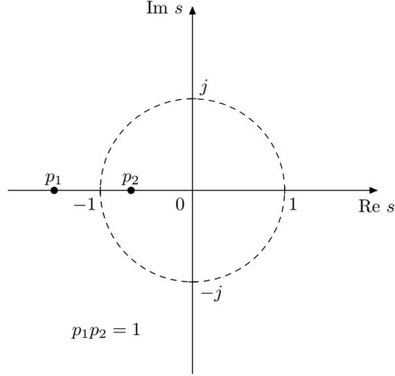
Figure 4.9: Poles of a non-resonating 2-pole filter ( $\omega_c = 1$ ).
