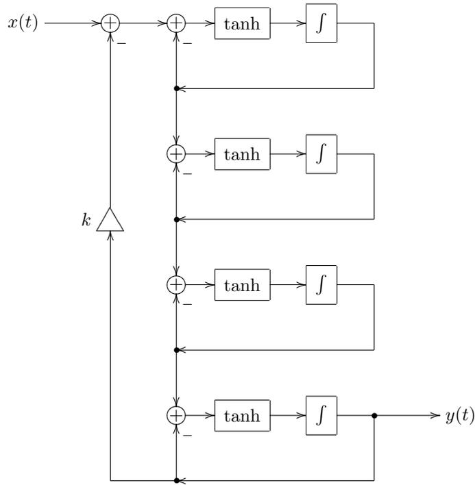
Figure 6.42: Flattened OTA lowpass ladder filter structure.
