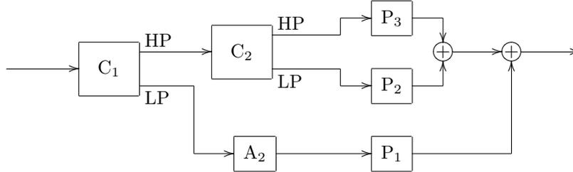
Figure 10.21: Phase correction in 3-way crossover mixing.
