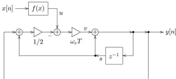
Figure 6.71: Structure from Fig. 6.70 with merged  $z^{-1}$  elements.
