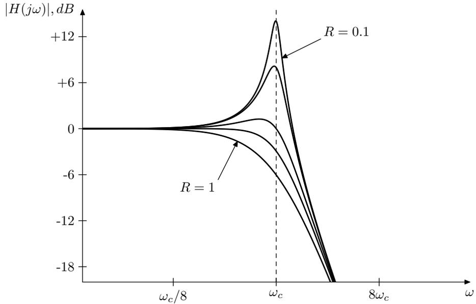
Figure 4.3: Amplitude response of a 2-pole lowpass filter.
