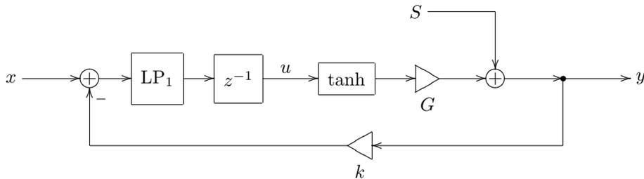
Figure 6.18: Using a 1-pole lowpass smoother to improve convergence of signals in Fig. 6.17.
