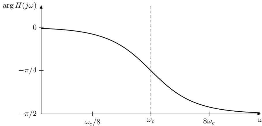
Figure 2.5: Phase response of a 1-pole lowpass filter.
