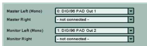
Optionally you can connect the left Master Left channel and the Monitor Left channel to hear both signals separately over your headphones (only in mono). With a standard dual
