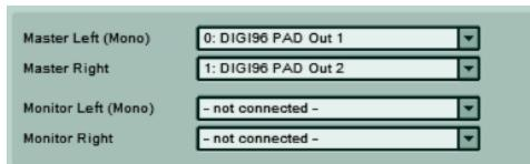
If you are running TRAKTOR with your onboard soundcard or a simple stereo soundcard we recommend to leave the monitor channel with the option **-not connected-**
