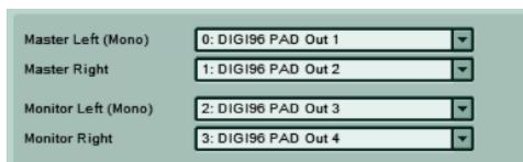
If you have a multichannel audiocard you should assign the master channel of **TRAKTOR** to the audiocard outputs that are used for amplifier connection. The monitor outputs should be connected to the headphone outputs of the audio card. We recommend to use an optional headphone amplifier.
