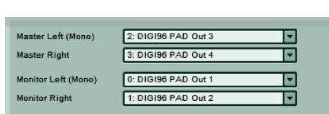
Many multichannel audiocards provide a separate headphone output that is identical to the outputs 1 and 2. In this case it is necessary to assign the **TRAKTOR** Monitor outputs to the outputs 1 and 2 of your audio card and the Master outputs to
